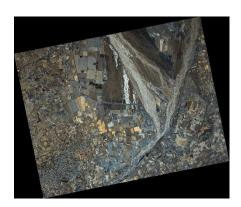
Acquisition by CSG2 Satellite on 21 February 2022 at 04:37 UTC. This is an acquisition in Spotlight-2B mode (0.6 m resolution on an area of 10x10 Km) made with double polarization (HH and HV). The combination of colors was obtained by combining the two polarizations with the average value between the two polarizations (RGB = HH, average, HV).
